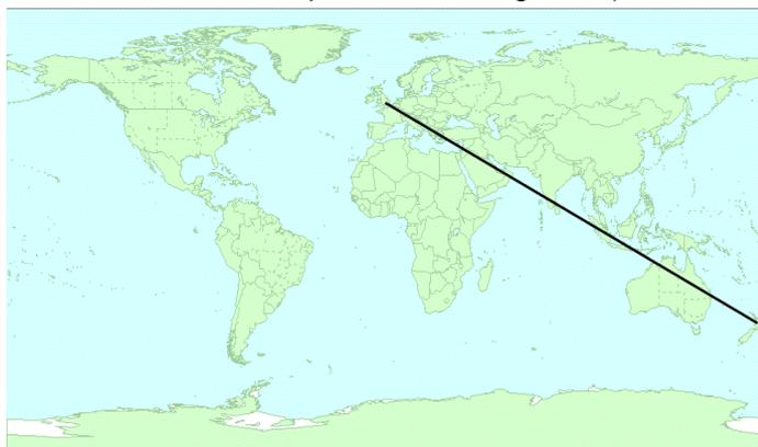
Mercator projection) will give you false information as to how the radio wave reaches it's target. To get the true picture you need to look at a globe or a special type of map called a '**GREAT CIRCLE**', which is a representation of the globe if it were flattened onto a piece of paper.
